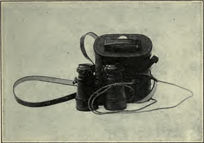
FIG. 31.—Type A. Showing the field glass and case with sling cord, shoulder straps, belt loops, and compass.
